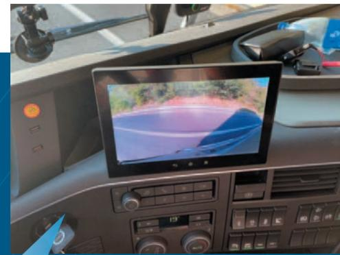
**The central screen** can also be used for viewing the image from the camera placed beneath the rearview mirror.
