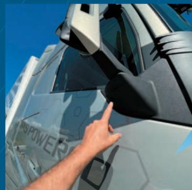
**And here** is the solution to replace the sticker: a camera that eliminates the blind spots.
